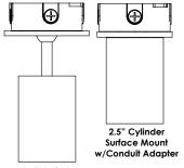
2.5" Cylinder Slope Pendant w/Surface Mount **Conduit Adapter**
