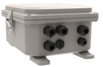
The **PDX-S** is an exterior-rated enclosure with a hinged cover that latches and seals using a formed in place PUR gasket and a stainless steel latch. It consolidates multiple input sources into two outputs to the ColourLine series fixtures. Data input from the RDM Color controller and AC input combine to provide output to two Starter Cords or two DMX Outputs. Splitter is fully RDM compliant.
